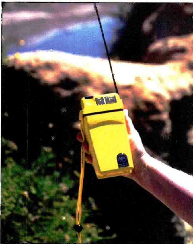
As long as the tape measure antenna has a "clear view" of the sky, the signals will reach the satellites.
