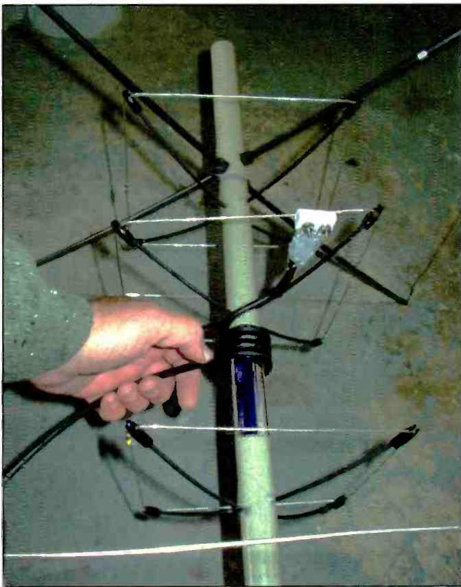
Winding the balun is easy with either RG58 or 9913 coax. Remember, at VHF and UHF frequencies you'll want to keep your coax run as short as possible to avoid signal loss.
