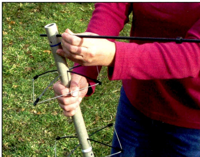
Assembling the antenna is quick and easy: just slide the spreaders into the boom's pre-drilled holes.
